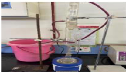
Fig (a): Experimental setup for Soxhlet apparatus
